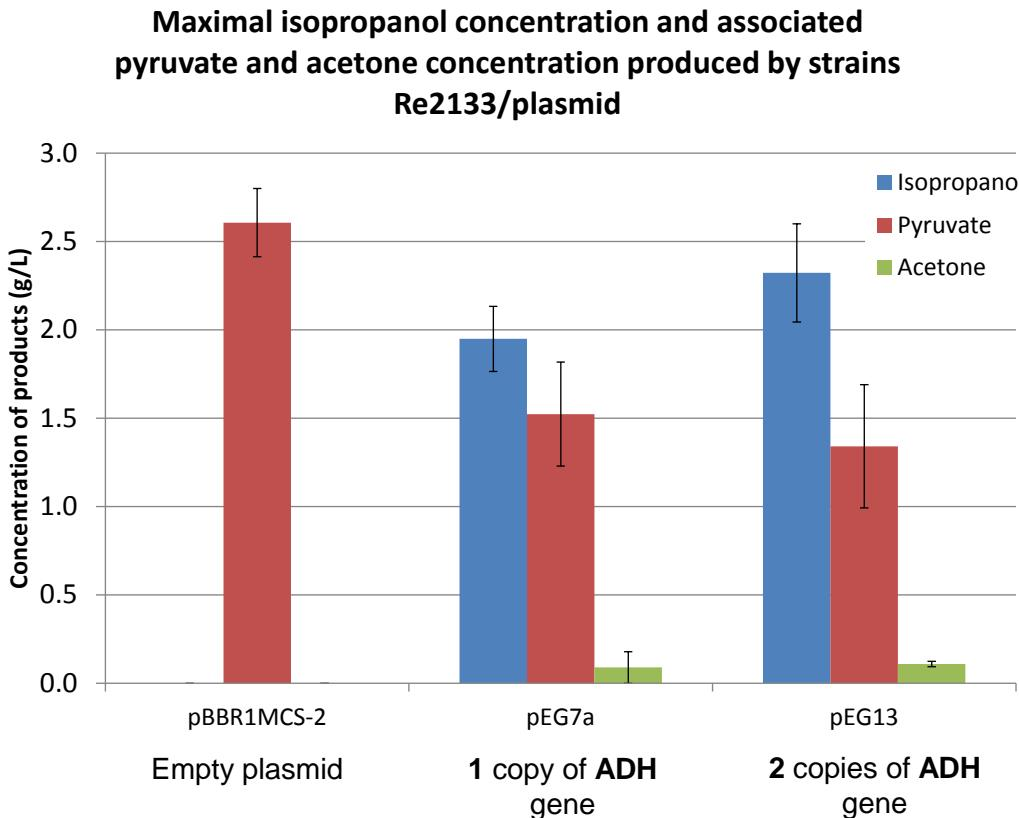
The Alcohol dehydrogenase is a limiting step for isopropanol production
